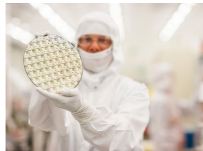
Imec was the world's first to develop 200V and 650V dispersion-free normally-off/e-mode power devices on 200mm Si Wafers.
