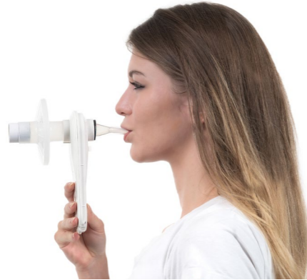
Prototype of imec's breathalyzer. It offers fast, easy and accurate identification of viral diseases that are transmitted by exhaled particles.
