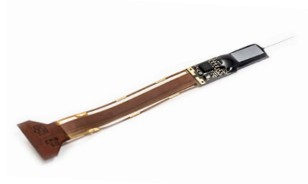
Neural probe enabling electrical and chemical recording and stimulation of single neurons.
